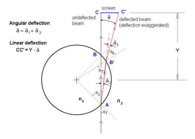
$n_1 \sin_1 = n_2 \sin_2$ The laser beam goes straight before pumping. With vacuum inside the beam gets deflected due to refraction Take \_1=45°. Solving this equation for \_2 we get \_2= 45.0166°.
