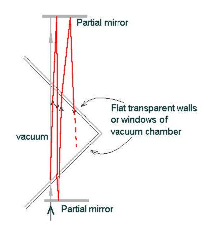
Repeated passage of the laser beam through a prism inside the vacuum chamber
