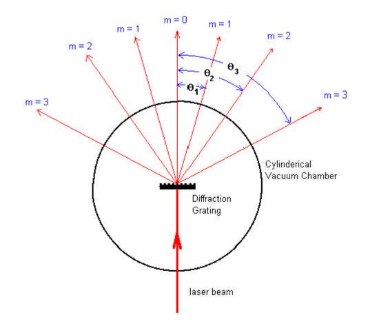
A laser beam is incident on the diffraction grating. The grating produces interference maxima on a screen. The angular position of a maximum (a bright spot on the screen) is given by the equation
