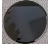
Figure 1. Film delamination caused by thermal non-uniformity
